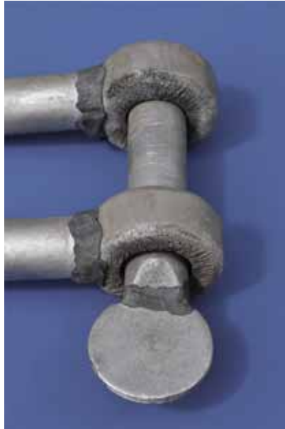
Figure 6.5: General corrosion in stainless steel shackle (4301) after a long period in a nitric acid/hydrofluoric acid-based pickling bath. Note that the whole item is corroded, but that the end surfaces of the steel bar and welds have been slightly more aggressively attacked than the rest.
