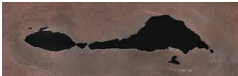
Figure 6.6: Molten salts at high temperatures may have the same effect on stainless steel as strong aqueous acids. This 6 mm thick base plate from an oven made of 4571 ('316Ti') has in just two years suffered from penetration due to contact with a strong fluoride-based flux for the soldering of aluminium. The flux had a fluoride content of up to 50%, and the temperature has been approx. 550°C.
