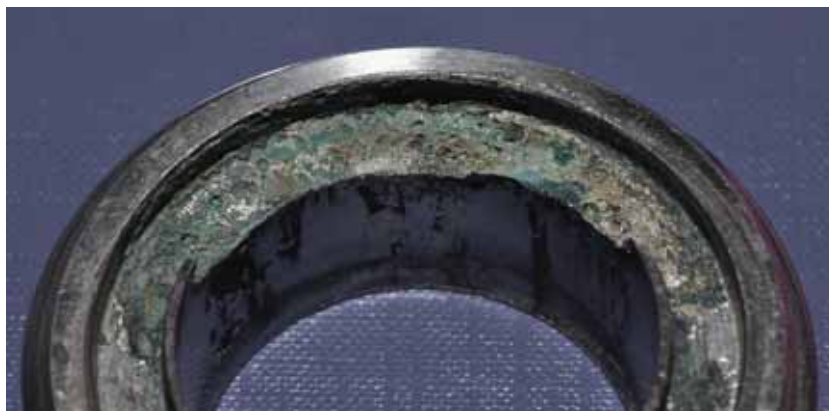
Figure 6.19: Crevice corrosion in a welding nipple of 4404 exposed to an aqueous solution of copper chloride ( \text{CuCl}_2 ). Note that the corrosion is concentrated in the seal track.
